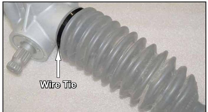
**Rack and Pinion Installation:** Do not tighten hardware completely unless noted.
