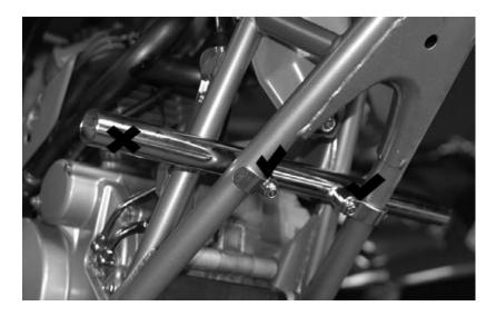
3. Slide the left side nerf bar on the front mount bar. Line up the outside hole on the rear nerf bar mount with the hole in the footpeg. Insert a bolt and lightly tighten a lock nut. Repeat this for the right side
