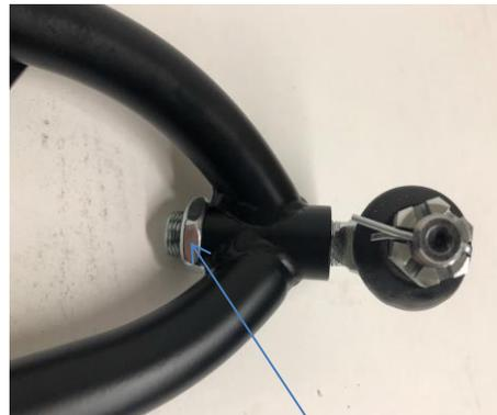
This is a lower a-arm. The nut for the ball joint goes on the back side of the arm.
