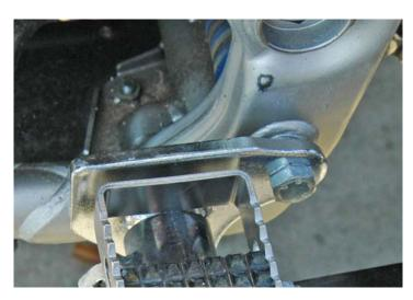
3) Install the forward nerf mounts. (see pic 2) Use the supplied short bolts and 1 spacer on each side. These mount in the forward lower engine mount bolt hole (remove the stock bolt, which you will not re-use). Do not tighten the bolts yet.
