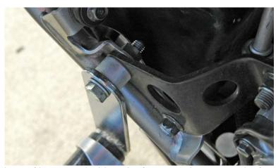
4) Install the nerf bar on each side. The foot peg tube goes on the foot peg mount and the forward tube goes over the forward mount tube.
