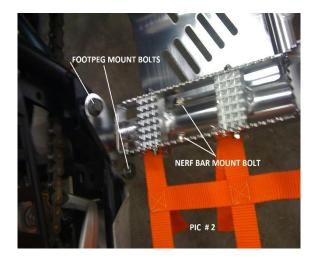
2. Remove the upper engine mount bolt and set aside. See Photo. Install front Pro-Peg Mount and long bolt with nylock/washer <u>but leave it loose</u> <u>for now!</u> You should be able to move the front mount at this time. It will make the install of the nerf easier.
