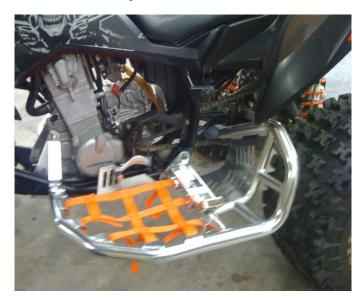
4. Now use the M6 bolts, Nylocs and Washers to attach the rear of the heel guard to the stock fender. The washer goes on the nut side.
