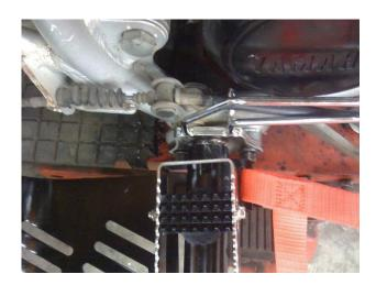
4. After you have confirmed all your hardware is installed and torqued to spec. Take your Blaster for a ride. When you get back re-torque ALL OF THE HARDWARE. This is REQUIRED!!! Re-check every few rides!!!
