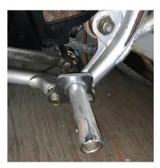
2. Remove the upper engine mount bolt and set aside. See Photo. Install front Pro-Peg Mount and long bolt with nylock/washer <u>but leave it loose for now!</u> You should be able to move the front mount at this time. It will make the install of the nerf easier.
