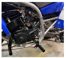
2. Install the brake side foot peg mount. Install the brake pedal to the pin on the foot peg plate, use grease on the pedal bushing. Make sure the circlip is seated in the groove on the pin. Use the stock bolts to attach the foot peg mount to the frame. Tighten to the Yamaha suggested torque setting.
