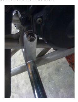
3. Slide the Nerf Bar over the front and rear mounts, adjust the front mount as needed. Use the rear mount #8 bolt and Nylocs to fasten the nerf bar to the peg. It crosses through the tube (See the first photo for reference) to hold the nerf bar to the peg. After you have confirmed alignment of the nerf bar, tighten the engine mount bolt to OEM spec and tighten the front clamp to 6LBS.
