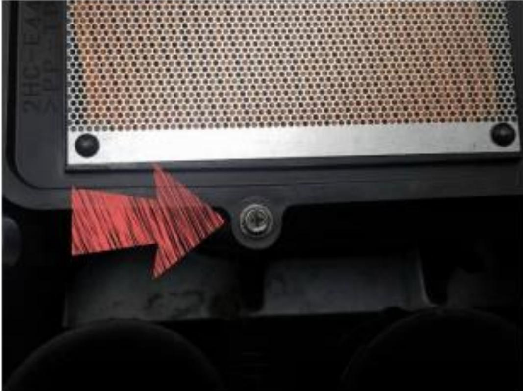
7. Install the provided 10mm bolt and rubber washer in the center position on the filter cover. Slide on the provided std washer and nylock nut and torque to 66 in/lbs.
