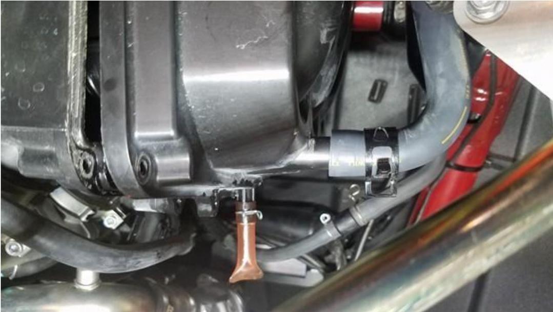
5. Carefully remove the filter cover pulling down from the bottom. The cover will make contact with the rubber air horns and you may have to manipulate it over them a bit. They are rubber.
