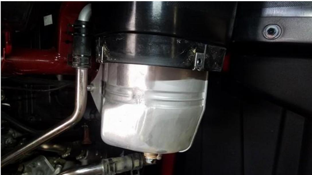
3. Use a combination of the ¼" drive ratchet, 3" extension, swivel extension, and 8mm socket to remove the 10 outer screws retaining the secondary filter cover and the hidden 1 screw recessed in center of cover.
