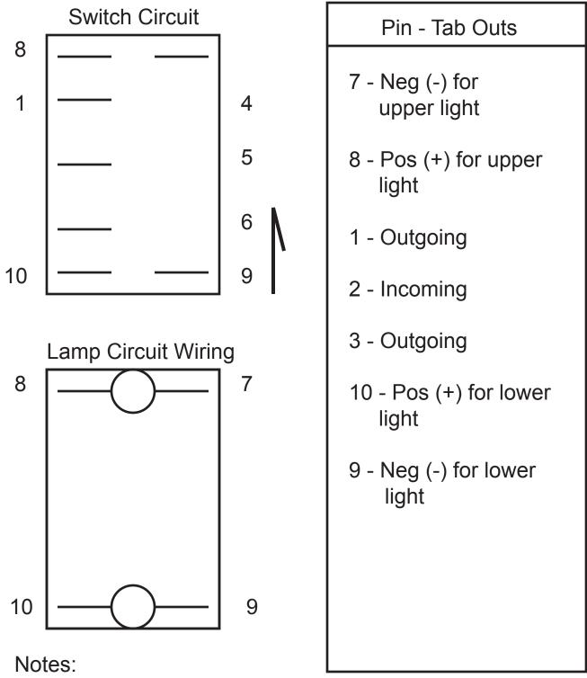
This is a dual lighted switch. Both lights in this switch are wired to be independent of the switch operation.
