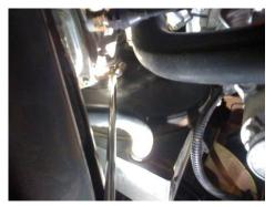
Now you need to remove the two clamps retaining the airbox to the throttle bodies. They are most easily accessed through the passenger side rear fender well. A longer screwdriver really makes this easier. Make sure you get both clamps.
