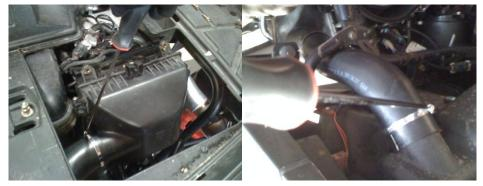
Remove the two clamps holding the rubber tube connecting the airbox to the resonator chamber in the left rear fender. Completely remove the rubber hose and clamps. We will not be re-using these.
