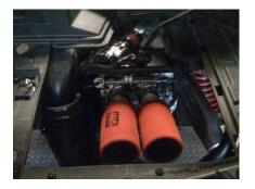
Don't forget to oil your filters before use. Proper cleaning and fitment will extend filter life and prevent engine damage. If you have any questions during the installation process feel free to give us a call at 858-486-4380.
