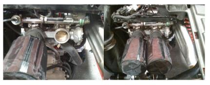
With the stock clamps installed on the Pod filters install them 1 at a time on to your throttle bodies. Pay attention to how you clock your clamps so you can access them easily.
