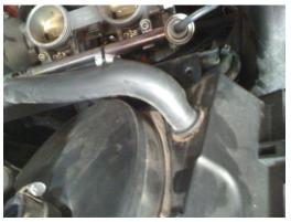
When you pull away the airbox there will be another hose connected to the back. Don't forget to disconnect it by gently pulling on it.
