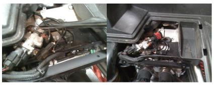
Almost finished. Remove the clamp and hose that is connected to the Idle air control valve. You will not be re-using this hose or clamp. Install the provided breather filter and you are finished.
