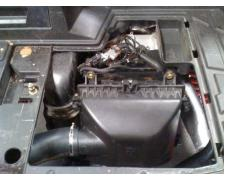
Begin by removing the engine cover to access the factory airbox.
