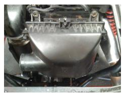
You should now have the bolts removed and the rubber hose removed and it should look like this.
