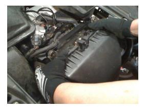
Gently pull the airbox away from the throttle bodies. It helps to use your fingers to slip the boots off of the throttle bodies. You shouldn't have to pull very hard. If it doesn't come off smoothly; loosen your clamps more.
