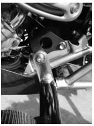
2) Mount the chrome bar mounts into this hole. Use the allen head bolts in the following sequence: Do not tighten the bolts yet!
