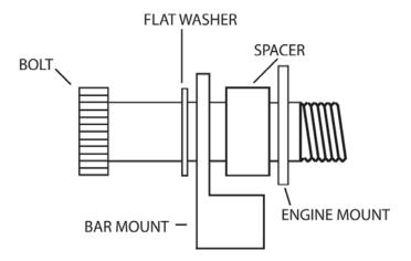
3) Slide the front tube of the nerf bar onto the bar mount. Line up the rear nerf mount bracket holes up with the holes in the foot peg and install the bolt then the washer and nut. You may tighten these nuts now as well as the front allen bolt. (See picture)
