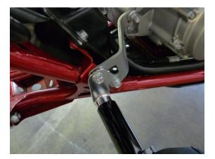
3) Mount the shifter side nerf bar peg mount (it has an "L" stamped on the back) Use the stock bolts with locktite. Tighten to 56 ft. lbs. of torque. (See pic 2)
