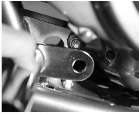
2) On both sides of the quad, loosely mount the chrome tube with the tabs facing backwards using the included hardware. (see picture)See photo below for assembly order. Make sure that the spacers are in the correct position between the chrome mounting hole and the frame.
