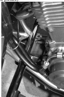
Note: The bar will go under the water and oil lines. Be sure you don't pinch the reverse cable under the mount bracket. Do not tighten the bolts yet!
