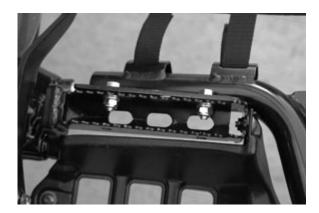
4) Tighten the foot peg bolts first, then tighten the engine mount bolt.
