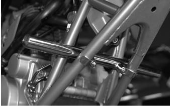
2. Cut off the plastic heel guard as shown in pic 2. Unbolt the piece that is left attached to the footpeg. Repeat for the other side.
