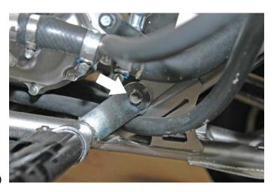
4) Mount the shifter side nerf bar peg mount (it has an "L" stamped on the back) Use the stock bolts with locktite. Tighten to 56 ft. lbs. Of torque. See Pic. 2:
