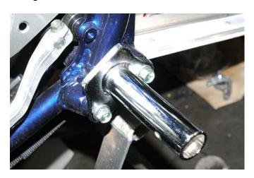
3) Install the forward nerf mounts. (see pic 2) Use the supplied long bolts and 1 spacer on each side. These mount in the forward lower engine mount bolt hole (remove the stock bolt, which you will not re-use). Do not tighten the long bolt yet.
