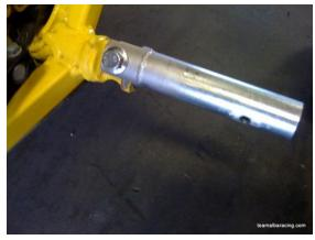
2) Install front mount as shown in picture. Use supplied spacers.
