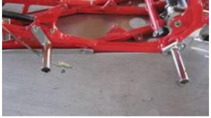
2) Install front mount as shown in picture. Use the supplied spacers between the mount and the frame. Use the supplied bolts. <u>Do not tighten the</u> <u>bolts yet.</u>
