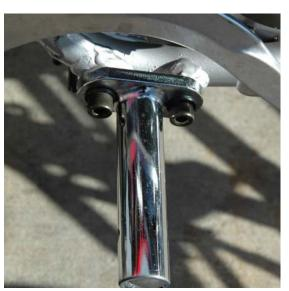
2) Mount the foot peg mounts to the frame (see pic 1) Note that there is a "L" and an "R" stamped on each mount. "R" goes on the brake side, "L" on the shifter side. Note that the tube is not welded centered on the flat bar. When you bolt these on mount them so the welded tube is on the low side of the bracket(towards the ground). Use the original bolts with locktite on them. Tighten them.
