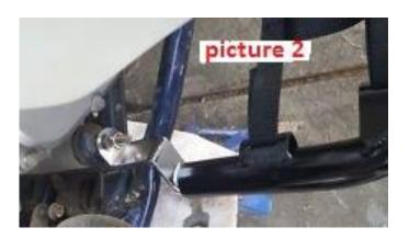
2) Use picture #3 and #4 as an example for mounting the nerf bars. Slide the front of the nerf bar onto the mount tube. Then hold the rear mount tab against the front of the footpeg. *Be sure the top edge of the mount is below the top of the footpeg teeth.* Use the supplied bolts, washers and nuts to mount the tab to the foot peg. Do **NOT** tighten these yet. Now repeat this procedure for the nerf bar on the other side of the quad.
