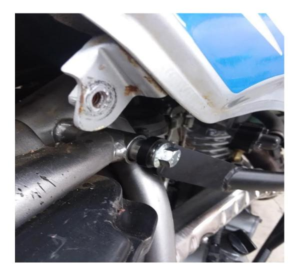
7. Install the front mounts. (Refer to drawing and picture below) Begin by installing the supplied 2 long bolts #1, 4 washers #2, 4 small aluminum spacers #5, 4 flange spacers #4, and 8 rubber isolators #3. Remove the 2 factory bolts for the front motor mount. You will reuse the factory nuts. Install per the diagram below. Do not fully tighten yet. It does help to have a second pair of hands here but it is not necessary.
