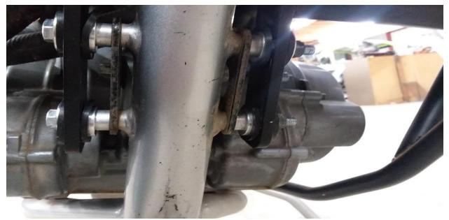
8. Install the lower mount. Use supplied mount #6 with supplied allen fasteners #7. Do not fully tighten yet.
