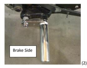
Step 3 — Unbolt the 2 bolts that mount the engine dampening rods to the frame. Lay the forward mount assembly across the frame and insert the 2 bolts. Do not tighten them. Refer to picture 3 (The quad is standing up in this picture)
