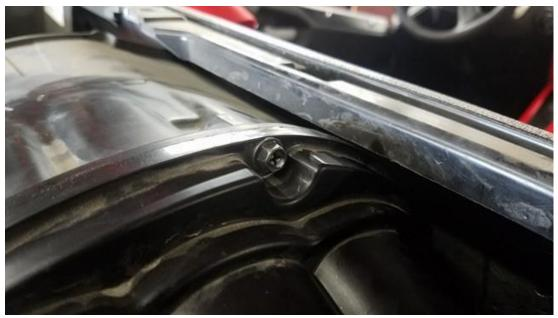
4.Using the pliers disconnect the breather hose attached to the bottom middle of the filter cover.
