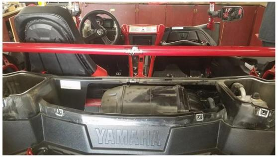
2.Using the ¼" ratchet and 10mm socket remove the oil tank cover.
