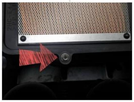
7.Install the provided 10mm bolt and rubber washer in the center position on the filter cover. Slide on the provided std washer and nylock nut and torque to 66 in/lbs.
