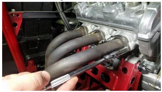
2. Using the 10mm socket and 3/8" ratchet loosen the header to muffler retaining clamp bolt. You will be re-using this clamp.
