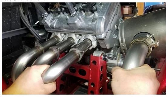
6. Loosely re-install the six 12mm nuts. DO NOT TIGHTEN THEM YET.
