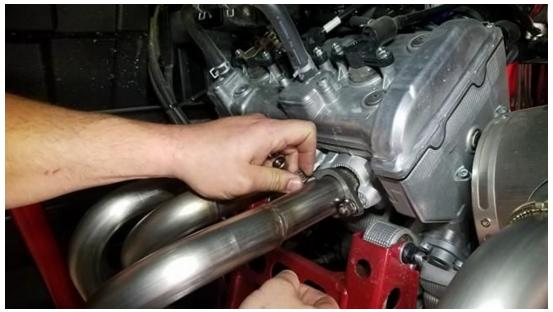
7. Loosely re-install the 10mm retaining clamp bolt.
