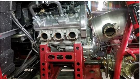
5. Install the new Alba Racing SBD Header. You may need to wiggle the header a bit to get it seated into the head and muffler.
