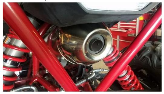
2. Begin by using the 5mm Allen wrench or Allen socket and ratchet to remove the muffler end cap retaining bolts.
