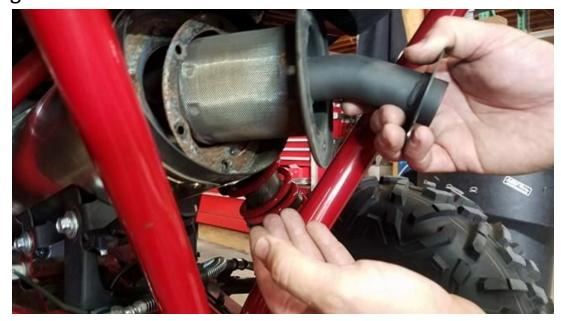
6. Move the OEM gasket over to the new Alba Racing Spark Arrestor and with 2 bolts in place install it into the back of the muffler loosely. Using 2 bolts will help keep the gasket in place while positioning.
