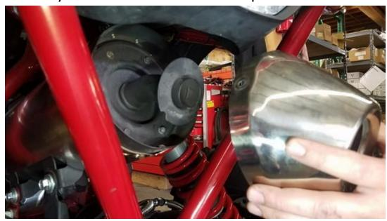
4. Using the 8mm socket, 3/8" drive swivel extension, 10" extension, and 3/8" drive ratchet carefully remove the six 8mm spark arrestor retaining bolts. These bolts have been known to break easily so take your time here. Some WD-40 may help.
