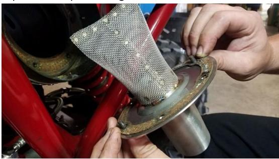
7. Loosely install and snug all remaining 8mm retaining bolts.
