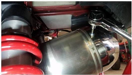
3. Carefully remove the muffler end cap.
